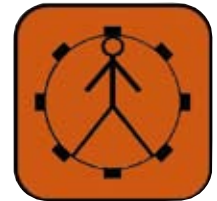
ENGINEER'S ALARM ENGINE ROOM
